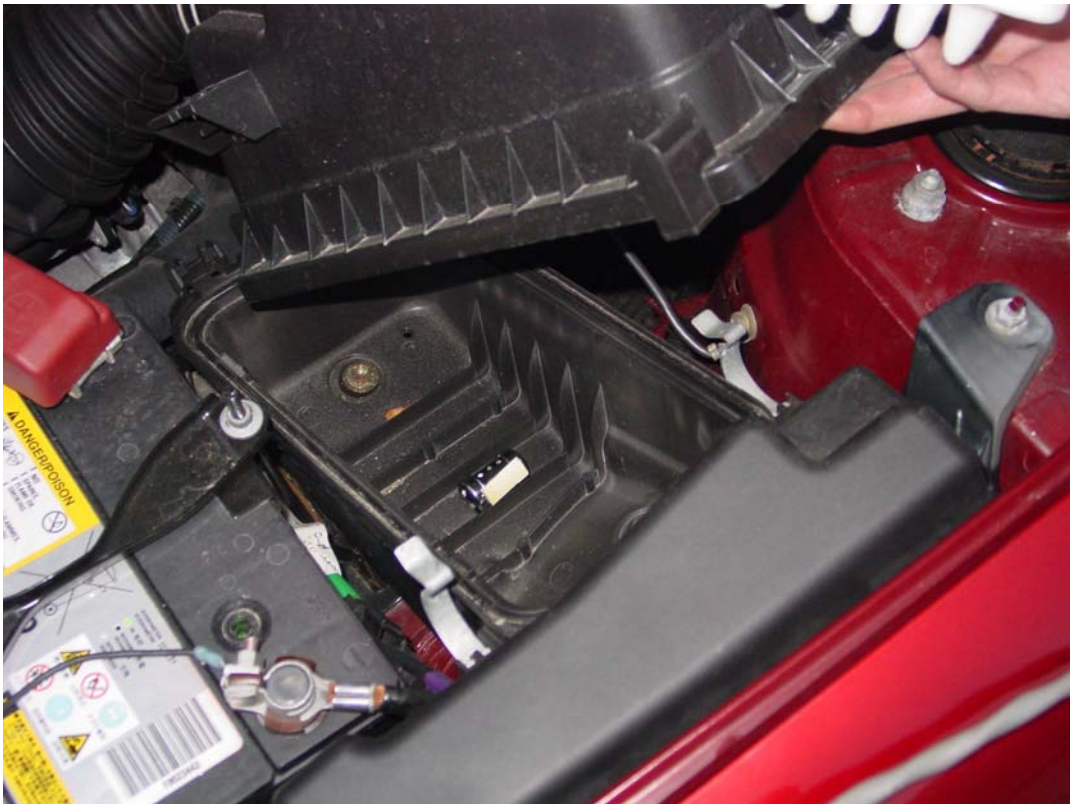
Modification Component Installed on Air Filter
