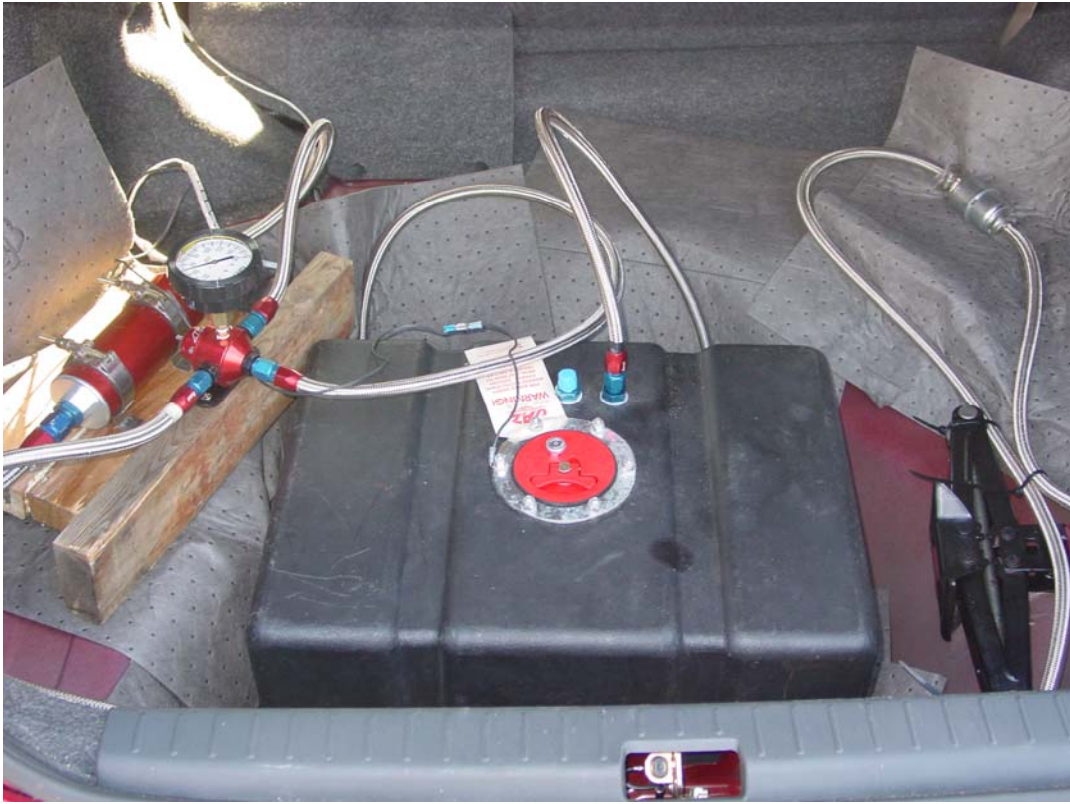
Portable Fuel System Setup
