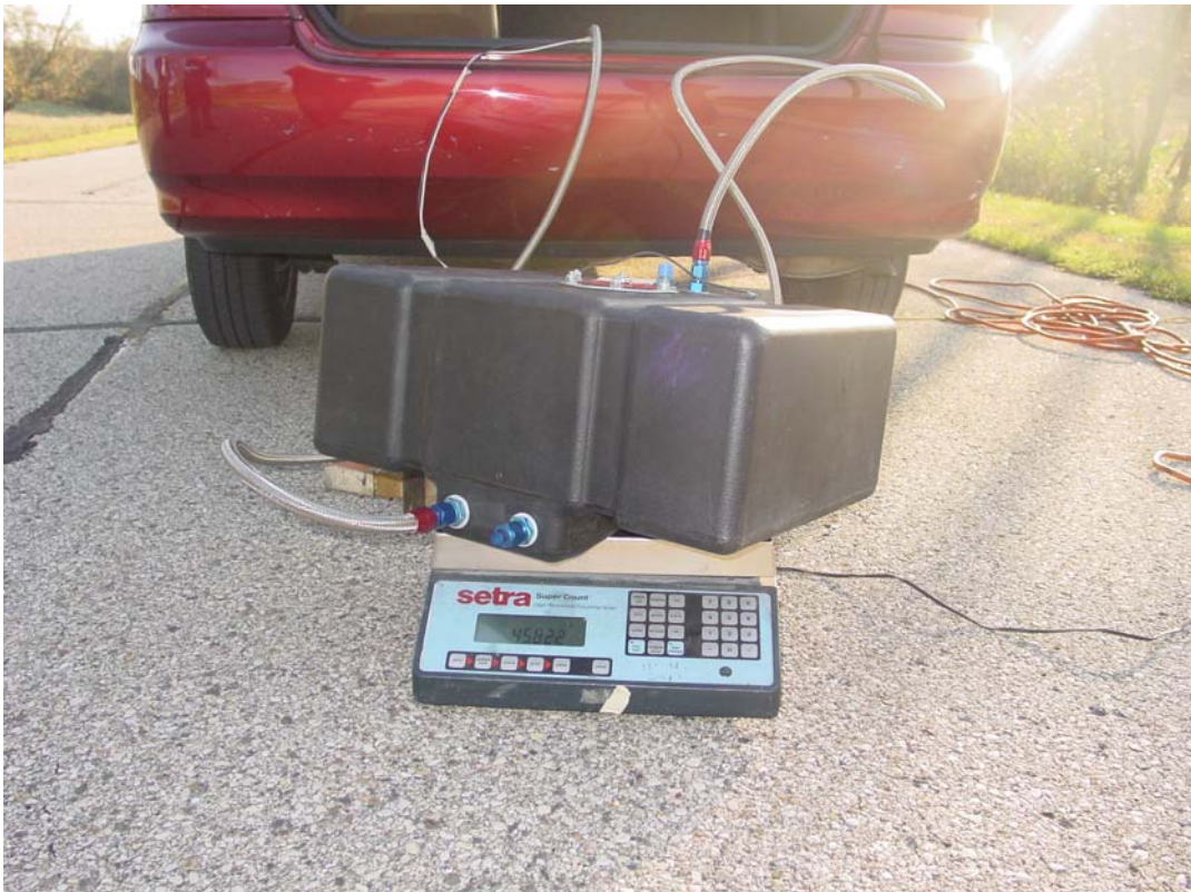
Fuel Tank Being Weighed
